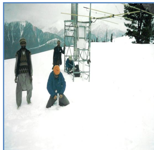
GMRC Team measuring Snow Water Equivalent (SWE) at Shogran in Kaghan Valley
